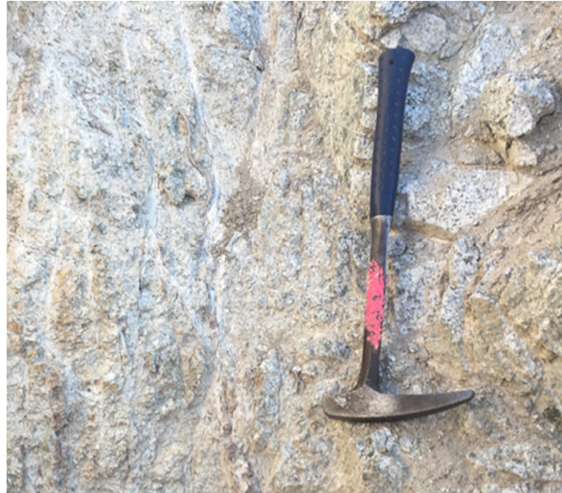
Shear zone in prospecting pit
